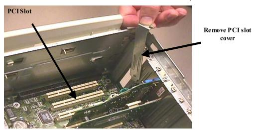
B-7 Carefully insert the Kingston® Ethernet Adapter into any empty PCI slot. Make sure the card is completely seated by pressing firmly.
